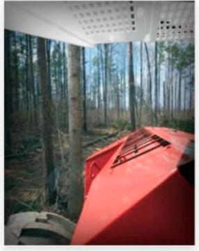
The engine housing is engineered with a sloped hood on each side to provide maximum rear visibility on both sides of the machine.
