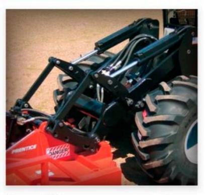
Rugged lift arms are constructed with a large torque tube and feature sealed pins and lift cylinders with cast ends for high durability.
