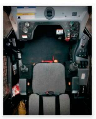
Joystick steering controls are available as an option for operators that prefer this type of machine controls. The joystick control system features the same fast cycle times with smooth control of all steering operations.
