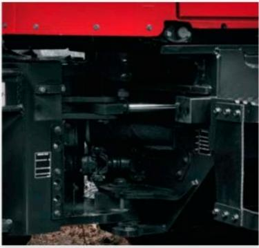
The center joint features large, double tapered roller bearings to provide years of trouble-free service in the rugged conditions of day-to-day harvesting.
