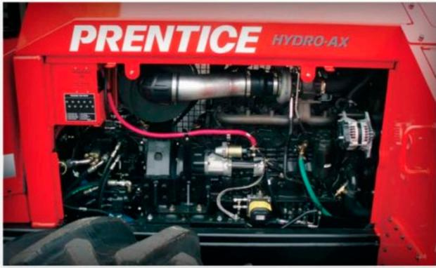
Screen doors on each side of the machine protect the engine compartment while in operation. The screens can be quickly removed to gain unobstructed access to the engine compartment for routine maintenance.
