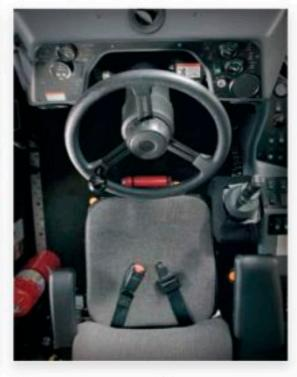
Operator comfort directly effects day-to-day productivity. Climate controlled Prentice operator stations maximize operator comfort while providing key features like "Quick-Steer" quarter-turn steering that dramatically improves cycle times while reducing fatigue.
