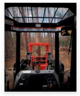
Triple laminated Lexan windows and skylight provide protection for the operator. The oversized windows give the operator an unobstructed view of work area.
