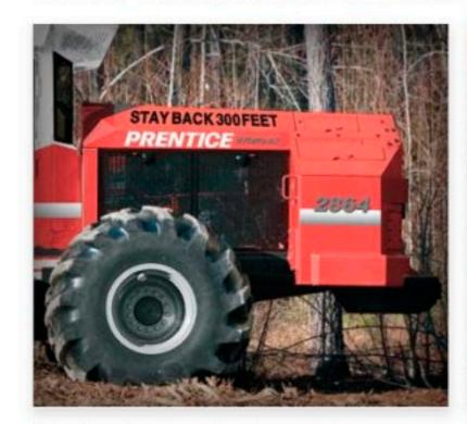
The Prentice engine house features angled panels to prevent debris from accumulating on the machine. Locking service covers provide quick and convenient access to the engine compartment. An optional bolt-on rear canopy is available.
